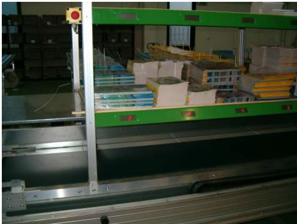
DGS Equipped shelves, one cell for each customer.
